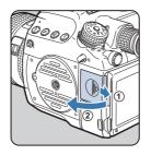
Insert the card all the way into the memory card slot with the memory card label facing toward the monitor.
