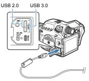
4 Connect the USB cable to the USB port of the computer.
