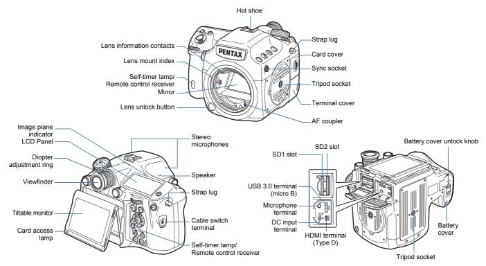
\* The front and rear views show the camera with the Hot shoe cover  $F\kappa$  removed.
