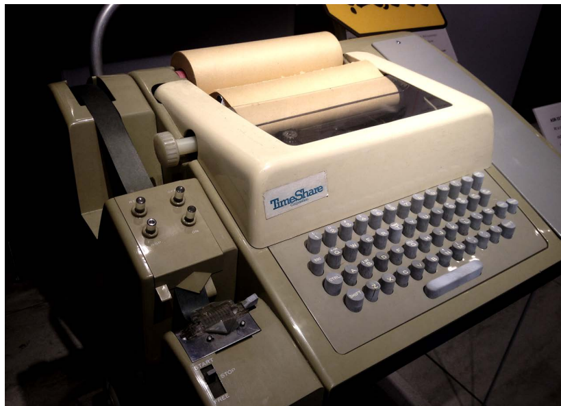
Figure 1-21: Teletype Computer Terminal with Attached Paper Tape Punch/Reader
