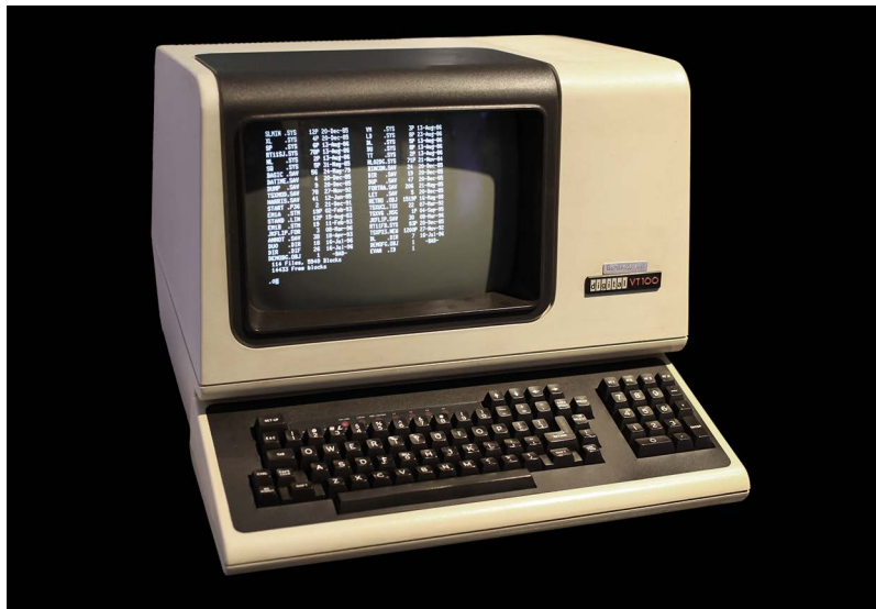
Figure 1-22: DEC VT100 Intelligent Terminal
